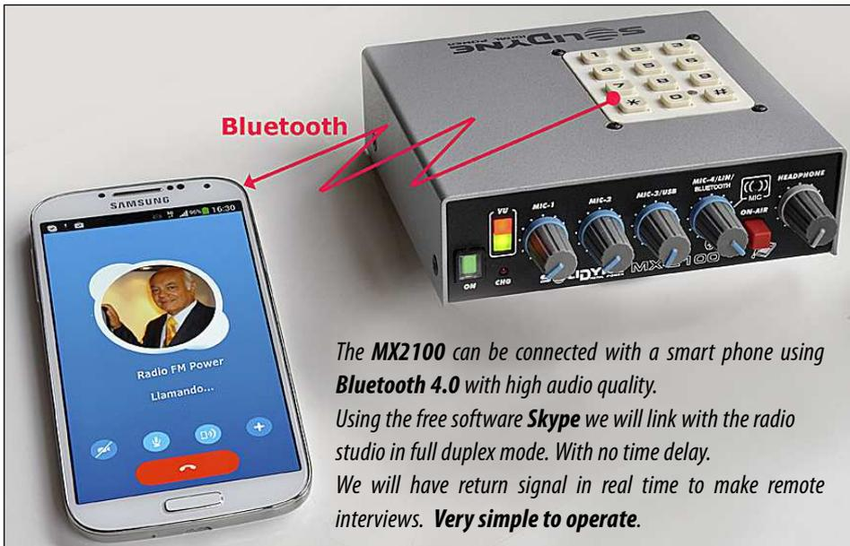
The MX2100 can be connected with a smart phone using **Bluetooth 4.0** with high audio quality. Using the free software **Skype** we will link with the radio studio in full duplex mode. With no time delay. We will have return signal in real time to make remote interviews. **Very simple to operate.**
