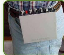
**A steel support** allows to use the console on the table or comfortably hung of your belt.
