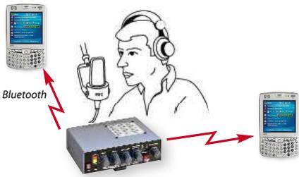
**The MX2100 provides wireless digital cell phone,** avoiding the use of cables and connectors.
