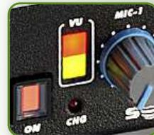
**The output level** adjustment does not require needle instruments because a simple indicator of two colors marks the level.
