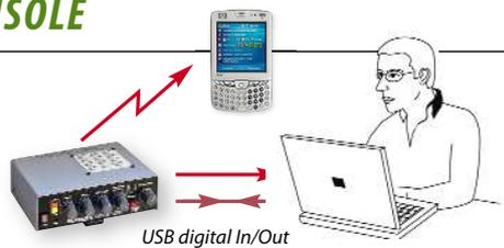
It has a **DIGITAL USB** connection to a Notebook. This allows the Internet transmission using a **3G/4 G** modem. You can use full duplex Skype, without delay, with high voice quality or generating a streaming **MP3 / AAC**.
