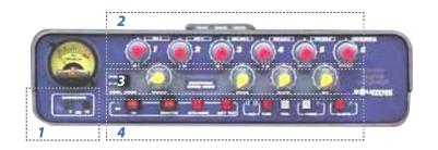
**2- Six stereo channels** transmission mixer manages mono and stereo audio.
