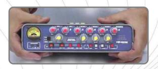
10 audio channels with digital output for stereo audio streaming.
