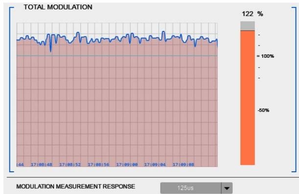
Figure 27: Modulation meter
