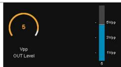
Change the MPX gain of the transmitter until achieve the desired modulation index on the 542's modulation meter (usually 100%). The default level for MPX output is 5 VPP. For fine tuning, change the MPX output level
