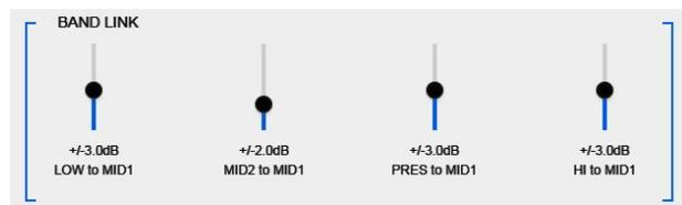
For music with vocal predominance and for microphones, the MB-AGC correction range should be narrow, about 2dB, except for the low band which can manage differences of 3 to 4dB (suitable values for balancing voices and materials with different bass levels).
