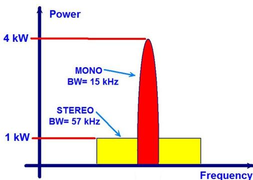
This technical advantage of monaural transmission can be exploited to combat interference, improving reception and radio coverage in times when talk shows must compete for the audience. The station can transmit mono at certain times and in stereo at other times.
