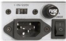
Before plugging the unit to the AC line, check if the 110/240V VOLTAGE SELECTOR is in the correct position. Use the supplied three-prong Interlok cable and ensure proper grounding.
