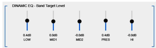
The maximum gain compensation applied is bounded by the "ACTION RANGE" control. The value indicates in dB, in each band, the maximum gain variation that will be applied to approximate the signal at the target level. For example:  $\pm 3\text{dB}$  limits the gain variation by 6dB, as the signal will be attenuated or increased by up to 3 dB as appropriate.
