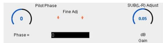
3. Repeat the measurement for the channel separation and check if the value increased. If instead of increasing decrease, go to the next step (4).
